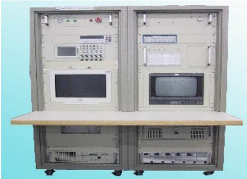
developed and became one of the **flagship product of the Group and its customer – Rafael Company**, Rafael uses the **Generic test equipment** for testing the Spike Missile system and its sub assemblies, many of which are classified. The generic test equipment is based on a **PC environment** and high quality connection zero force **Receiver interface (VPC)**. A combination of standard off-the shelf items, such as an industrial pc, which contains a variety of cards (A/D, D/A, DIO, etc.)
